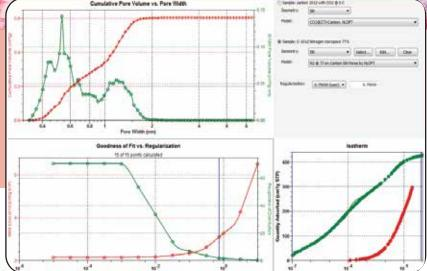
This advanced NLDFT method allows users to determine the pore size distribution of their sample using two isotherms. In this example CO2 adsorption (red) at 273 K and nitrogen adsorption (green) at 77 K are used to calculate a single pore size distribution. Users do not have to cut and paste distributions from CO2 and nitrogen – a single distribution is determined using both isotherms.
