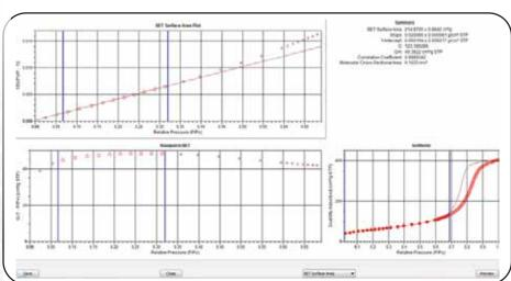
Calculations, such as the BET surface area transform plot, can be easily generated and adjusted. The selection bars allow for a range of data points to be quickly and easily selected. As a result, the summary of values derived from the calculations is instantly updated. Within the calculation window(s), the range of data used can be further refined.
