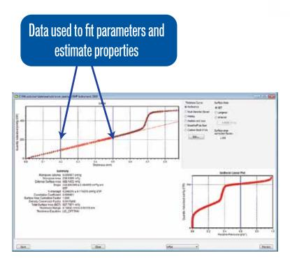
MicroActive interactive features reduce the often difficult trial-and-error procedure for fitting the t-Plot by providing direct feedback to the user.
